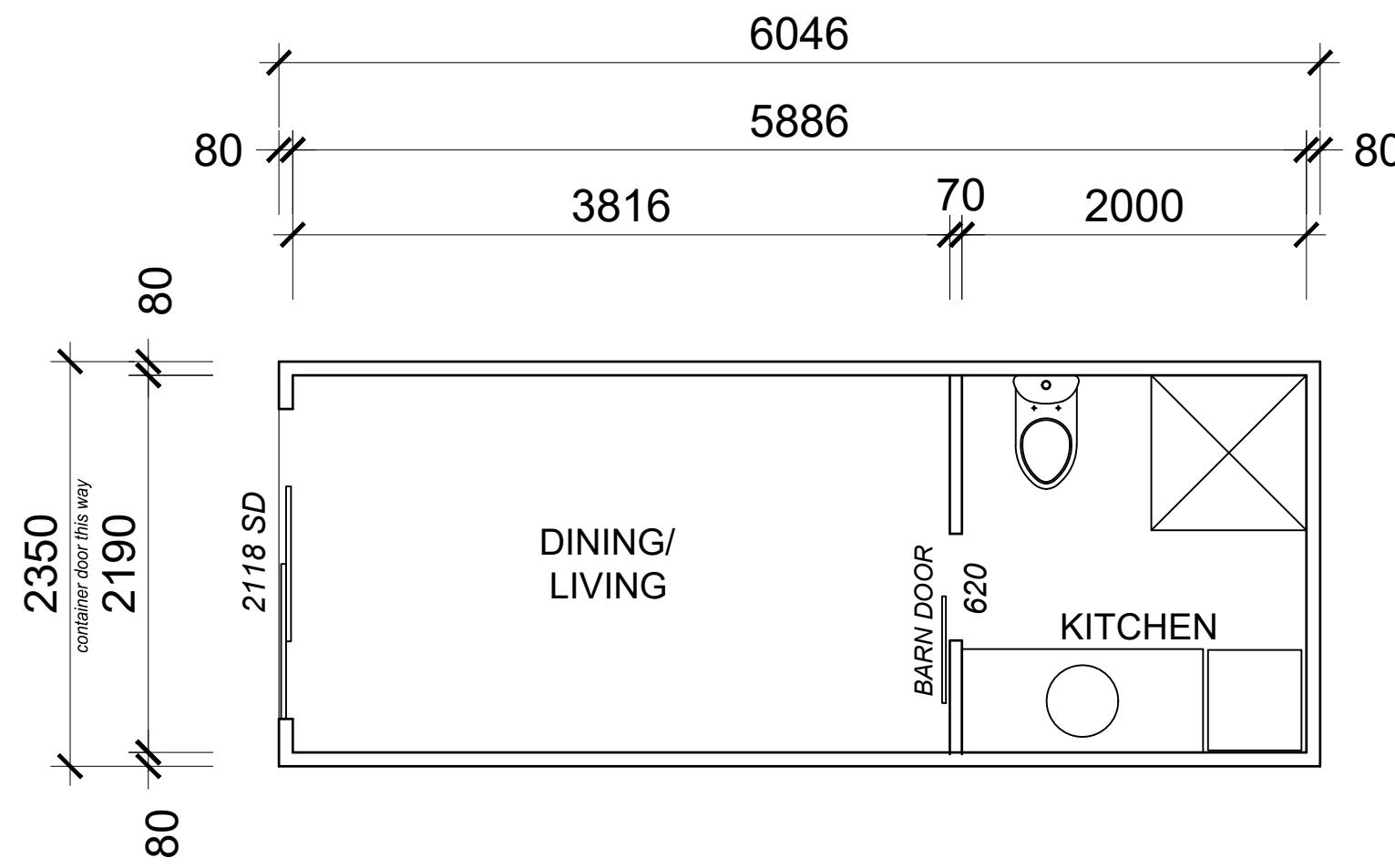
ALL CORNERS IN CONTAINER INTERNAL MUST BE CAULKED, THIS INCLUDES ANY WALL JOINS AND ARCS/ SKIRTS ETC. TO AVOID CRACKING
